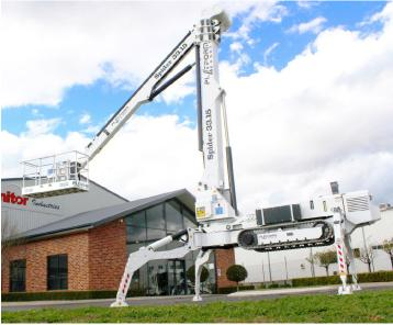
The 3315's unique telescoping articulated boom design provides exceptional up and over outreach specifications. Dual position stabiliser legs allow the 3315 to be set-up in the most difficult locations. Even with the stabilisers set in the narrow position, a complete 360 degrees slew is still possible!
